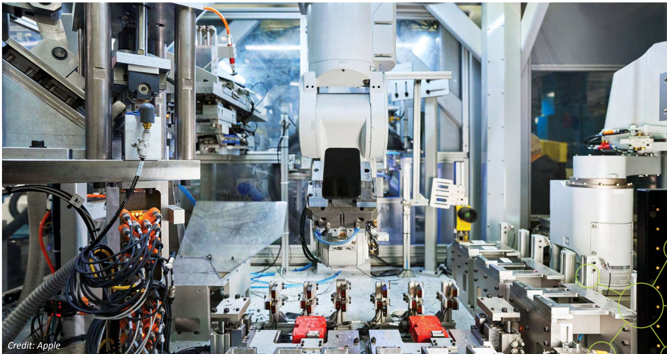
Apple's Daisy, which can disassemble up to 1.2 million phones each year to help recover valuable materials for recycling.
